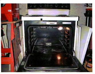
I took out the racks and made a bunch of removable hooks that parts can be hung from. The racks can be used for things like wheels that you can powder coat while on the rack and then place in the oven.
